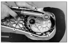
Make sure that the shafts can rotate.
